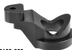
C-00180-266 Servo Saver Steering Arm - Aluminium 7075 T6 - Hard Anodised - Black - 1 pc
